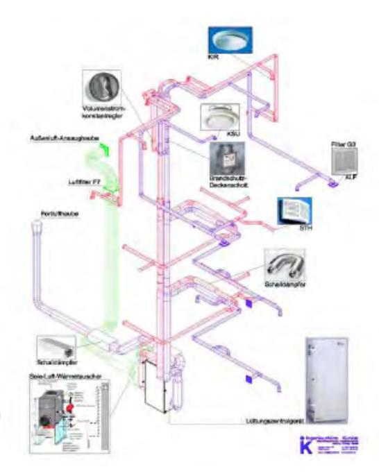
Heatpump and ERV in tight spaces integrated vertically
